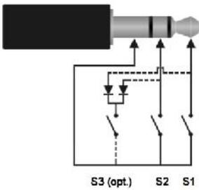
**Note:** There is no industry standard for which switch (Left, Right) is connected to the Tip and Ring on commercially-available foot pedals. This manual only refers to the 'Tip switch,' 'Ring switch,' etc.; and the actual response may often change between models/manufacturers.
